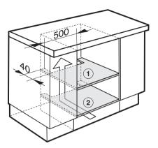
To ensure that the Combi Steam Oven has adequate ventilation, the following cut-outs measuring  $19 \ 11/16" \times 1 \ 9/16"$  (500 x 40 mm) must be made:
